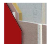
Isolation + structure bois + Bardage bois
